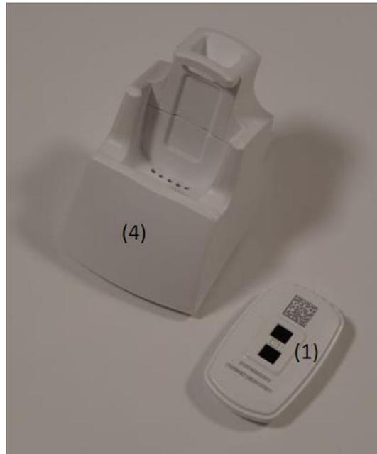
**A Base / Receiver (21)**, which must be connected to a USB port on the computer.
